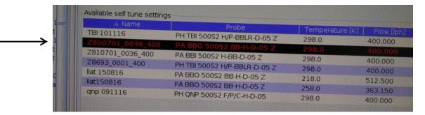
then click on Restore to Channel 1 button to load the self-tune parameter for room temperature operation. Click on ON button in the Temperature Tab of the Temperature Control Suite to turn on the VTU. Wait until the target temperature reaches and stabilizes at 298 K.
