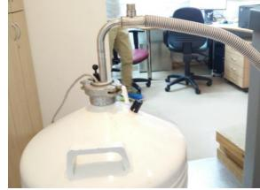
7. Attach the transfer line to the probe. Keep the transfer line horizontal when connecting the transfer line to the probe.
