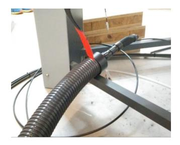
5. Connect the nitrogen transfer line cable to the LN2 box adapter (hidden under the black sponge to protect it from the humidity)
