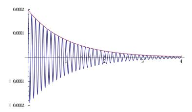
The voltage v(t) (blue line) decays with a time constant  $T_2$  and oscillates with a time constant  $\omega = \gamma B_0$ . The purple line is simply the exponential envelope:
