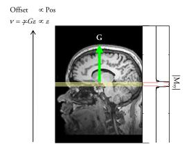
The gradient assigns frequencies to positions via  $v = \neq Gz$ , and hence any pulse that excites a range of frequencies  $BW = \neq B_1$  will, in the presence of a gradient, excite a range of positions given by:
