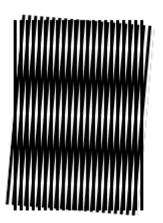
In k-space the illumination with a grating basically offsets the transmitted components through the objective by k of the grating (but in it the -k and +k as well as the DC component are mixed, so that several measurements are required to distinguish which observed component belongs where).
