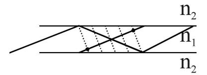
In considering the mode structure of waveguides we must solve for a self-consistent (phase matched) solution for a plane wave propagating at an angle to the waveguide. In doing this we have to take into account the phase shift following total internal reflection (remember polarization, beginning of semester).
