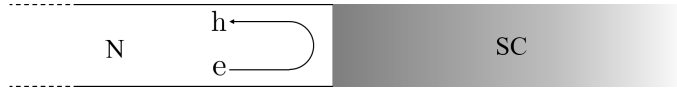
Figure 1.3: Andreev reflection of an electron into a hole at the interface between a normal-metal lead and a superconductor. When the superconductor is a topological superconductor, electrons (or holes) at the Fermi level experience perfect Andreev reflection.
