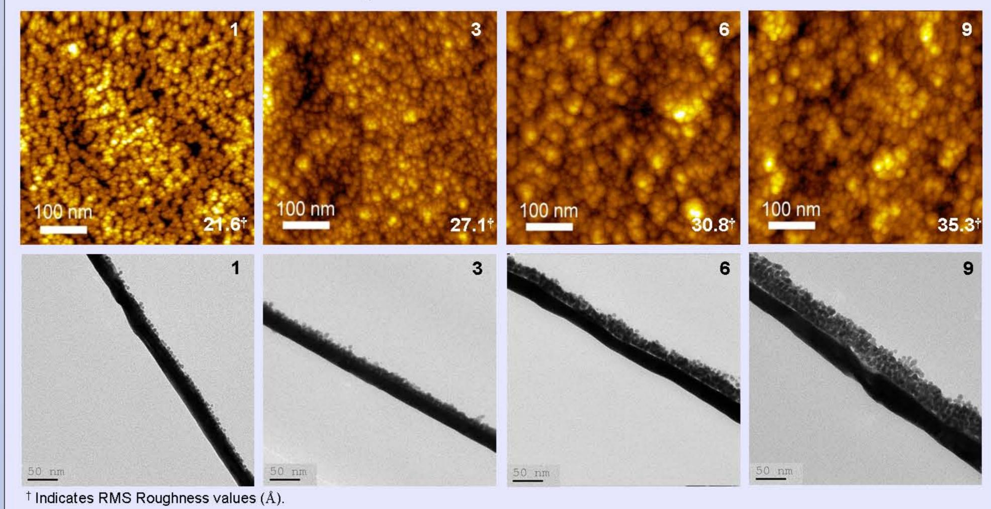
6. Vertical spacing of a NP layer from the gold surface using a coordinated organic multilayer.
