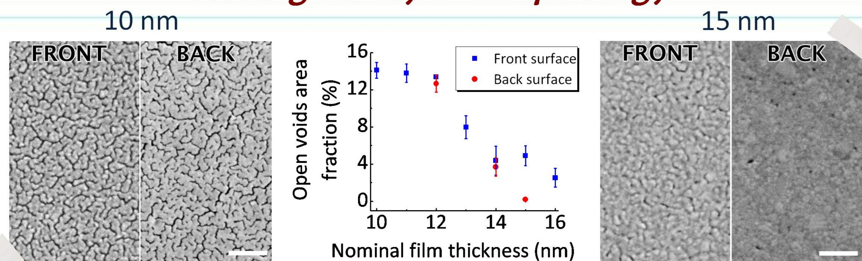
A 10-nm-thick evaporated Au layer shows open voids penetrating to the glass; a 15-nm-thick layer is asymmetric, showing continuous Au at the bottom.
