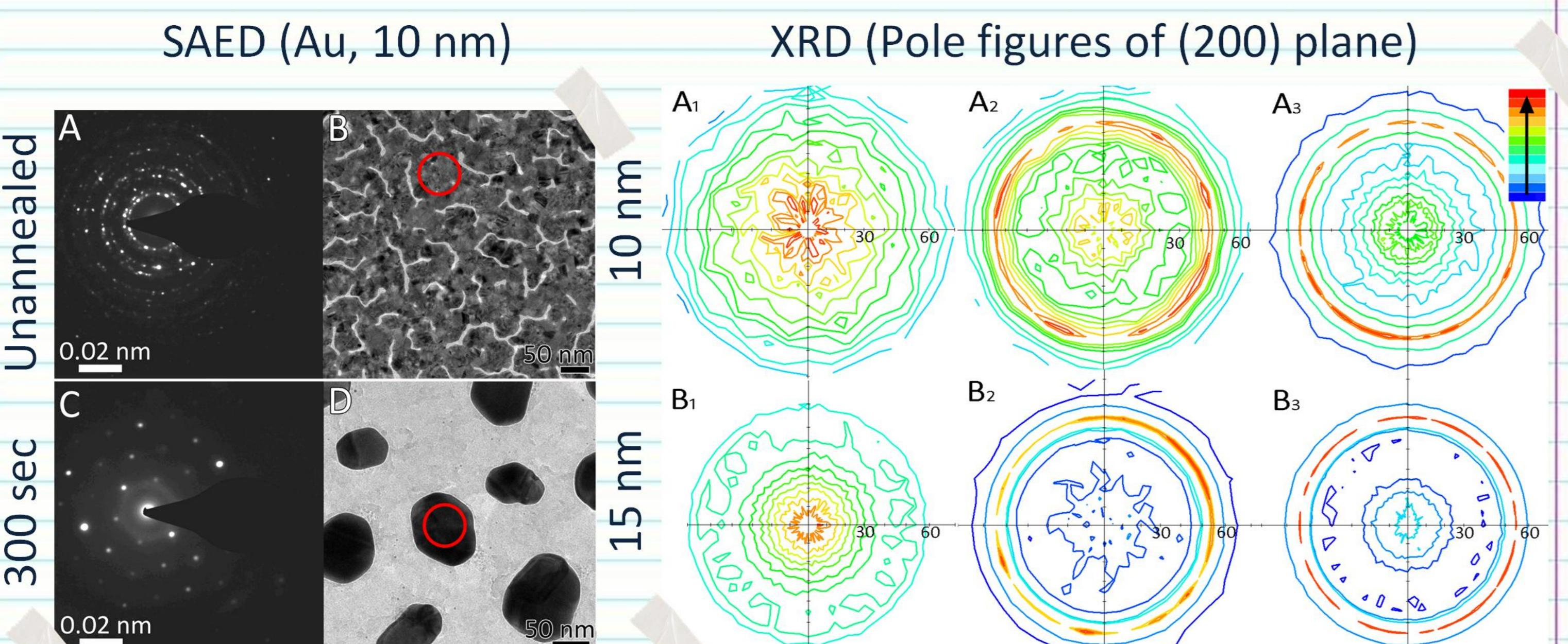
**Left:** Selected-area electron diffraction (SAED) and corresponding TEM images of a 10 nm Au layer, as-deposited and after 300 sec at 550 °C (red circle indicates the selected area aperture). **Right:** A representative set of pole figures obtained at the Bragg angle of {200} ( $\theta = 44.4^\circ$ ). (A<sub>1</sub>, B<sub>1</sub>) as-deposited Au layers on bare glass; (A<sub>2</sub>, B<sub>2</sub>) 300 sec and (A<sub>3</sub>, B<sub>3</sub>) 10 h at 550 °C.
