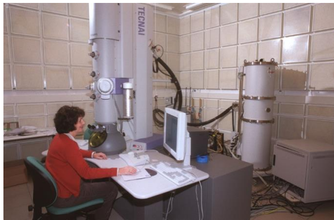
Figure 11. Dr. Ronit Popovitz-Biro at work with the high-resolution F30 TEM. Note the acoustic noise shielding on the walls and the cylindrical power-supply tank delivering 300 keV
